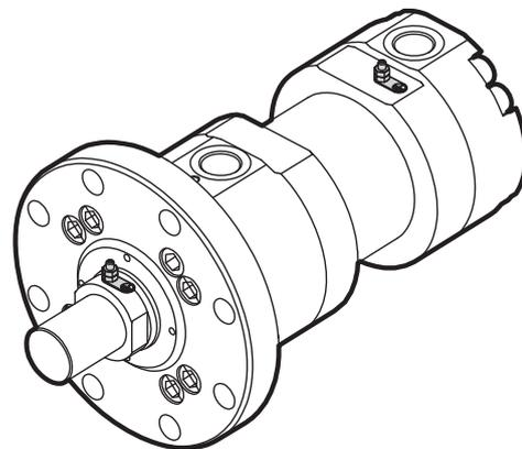
The bottom grounding point must always be connected whereas the connection of the rod grounding point can be avoided in case the whole mechanical stroke is covered during the cylinder operating phase (from the mechanical stop on the cylinder head to the mechanical stop on the bottom), or in case the rod has already been grounded through the mechanical connection between the rod itself and the machine/plan it is installed on.
