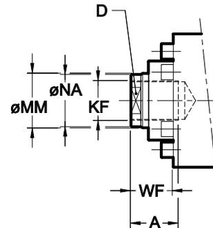
\* For bores  $\varnothing$  180 (piston rod  $\varnothing$  110) and higher, the rod has 4 holes at  $90^\circ$  realized on  $\varnothing$  NA and of  $\varnothing$  shown in the table.
