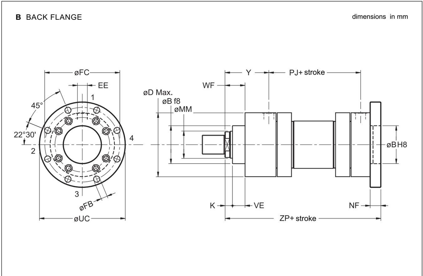
**NOTE:  $\varnothing 400$  bore has 12 equally spaced  $\varnothing FB$  holes in the mounting flange**
