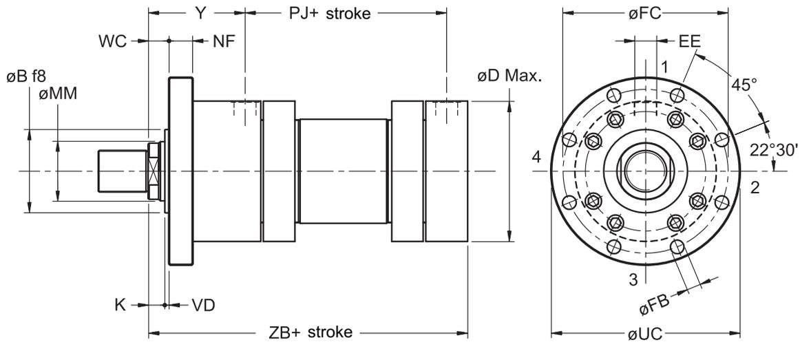
**NOTE:  $\varnothing 400$  bore has 12 equally spaced  $\varnothing FB$  holes in the mounting flange**
