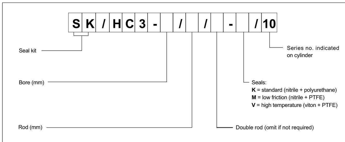
**NOTE:** the seal kit includes all the seals of a full-options cylinder (cushionings and external drain).
