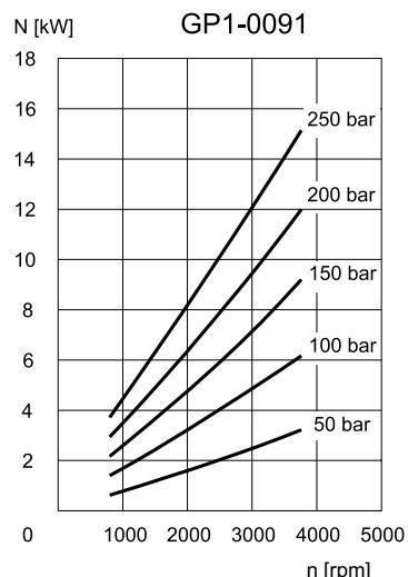
**5 - CURVES AND CHARACTERISTIC DATA OF GROUP GP2 PUMPS** (values obtained with mineral oil with viscosity of 36 cSt at 50°C)
